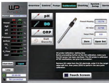
Online system calibration with system feedback
