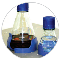
Snap shaker flask in clamp
