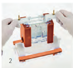
2 Transfer to casting base and tighten cams.
