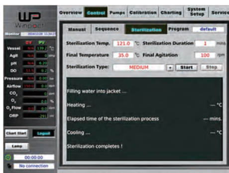
One-Touch automatic sterilization for vessel and system tubing
