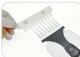
All combs are multichannel pipette compatible
