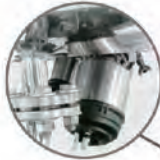
Harvest valve Sanitary level diaphragm type
